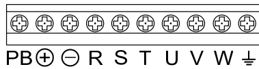
a) small and medium power terminal, part of the terminals slightly different
